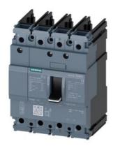
circuit breaker 3VA5 UL frame 125 breaking capacity class S 25kA @ 480V 4-pole, line protection TM210, FTFM, In=90A overload protection Ir=90A fixed short-circuit protection Ii=10 x In N conductor unprotected without connection
