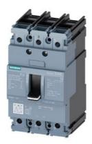
circuit breaker 3VA5 UL frame 125 breaking capacity class S 25kA @ 480 V 3-pole, line protection TM210, FTFM, In=90A overload protection Ir=90A fixed short-circuit protection Ii=10 x In cable connection on both sides
