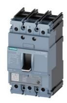
circuit breaker 3VA5 UL frame 125 breaking capacity class S 25kA @ 480 V 3-pole, line protection TM230, FTAM, In=90A overload protection Ir=90A fixed short-circuit protection Ii=5...10 x In UL489 SB (naval), 50 deg. cel. cable connection on both sides
