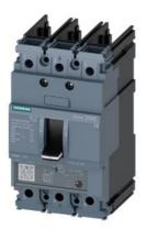
circuit breaker 3VA5 UL frame 125 breaking capacity class S 25kA @ 480V 3-pole, line protection TM230, FTAM, In=90A overload protection Ir=90A fixed short-circuit protection Ii=5...10 x In UL 489 SB (naval), 50° C without connection
