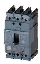
circuit breaker 3VA5 UL frame 125 breaking capacity class S 25kA @ 480V 3-pole, line protection TM230, FTAM, In=90A overload protection Ir=90A fixed short-circuit protection Ii=5...10 x In without connection
