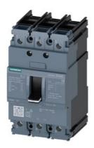
circuit breaker 3VA5 UL frame 125 breaking capacity class H 65kA @ 480 V 3-pole, line protection TM210, FTFM, In=125A overload protection Ir=125A fixed short circuit protection Ii=10 x In box terminals
