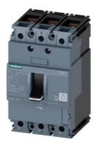
circuit breaker 3VA1 IEC frame 160 breaking capacity class N Icu=25kA @ 415V 3-pole, line protection TM210, FTFM, In=16A overload protection Ir=16A fixed short-circuit protection Ii=20 x In nut keeper kit
