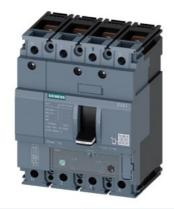
circuit breaker 3VA1 IEC frame 160 breaking capacity class M Icu=55kA @ 415V 4-pole, line protection TM240, ATAM, In=80A overload protection Ir=56A...80A short-circuit protection Ii=5...10 x In N conductor protection 100% nut keeper kit
