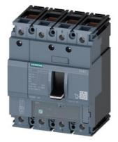
circuit breaker 3VA1 IEC frame 160 breaking capacity class N Icu=25kA @ 415V 4-pole, line protection TM220, ATFM, In=160A overload protection Ir=112A...160A short-circuit protection Ii=10 x In N conductor protection 50% clamp connection
