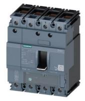
circuit breaker 3VA1 IEC frame 160 breaking capacity class S Icu=36kA @ 415V 4-pole, line protection TM220, ATFM, In=125A overload protection Ir=88A...125A short-circuit protection Ii=10 x In N conductor protection 50% clamp connection
