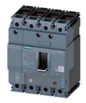
circuit breaker 3VA1 IEC frame 160 breaking capacity class N Icu=25kA @ 415V 4-pole, line protection TM240, ATAM, In=125A overload protection Ir=88A...125A short-circuit protection Ii=5...10 x In N conductor protection 100% nut keeper kit
