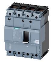
circuit breaker 3VA1 IEC frame 160 breaking capacity class N Icu=25kA @ 415V 4-pole, line protection TM210, FTFM, In=100A overload protection Ir=100A fixed short-circuit protection Ii=10 x In N conductor protection 50% nut keeper kit
