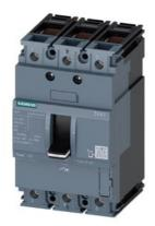
circuit breaker 3VA1 IEC frame 100 breaking capacity class N Icu=25kA @ 415V 3-pole, line protection TM210, FTFM, In=25A overload protection Ir=25A fixed short-circuit protection Ii=12.8 x In clamp connection
