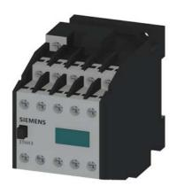
Contactor relay, 55E, EN 50011, 5 NO + 5 NC, 1U, screw terminal 24 V AC 50 Hz/29 V AC 60 Hz AC operation,
