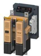
Contactor, Size 4, 2-pole, DC-3 and 5, 75 A Auxiliary switch 22 (2 NO + 2 NC) 400/380 V AC 50 Hz, 480/460 V 60 Hz AC operation
