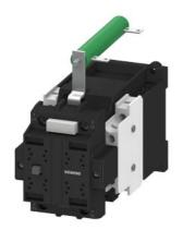
Contactor size 2, 2-pole DC-3 and 5, 32 A Auxiliary switch 22 (2 NO + 2 NC) DC operation 36 V DC
