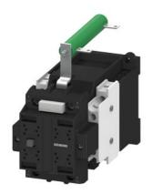
Contactor, Size 2, 2-pole, DC-3 and 5, 32 A Auxiliary contacts 22 (2 NO + 2 NC) 24V DC DC operation Operating range 0.7/0.8-1.2 UN
