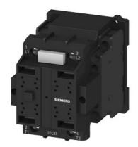
Contactor, Size 2, 2-pole, DC-3 and 5, 32 A Auxiliary contacts 22 (2 NO + 2 NC) 380/460 V AC 50 Hz/60 Hz AC operation
