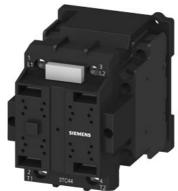
Contactor, Size 2, 2-pole, DC-3 and 5, 32 A Auxiliary contacts 22 (2 NO + 2 NC) 220 V AC 60 Hz/183 V AC 50 Hz AC operation
