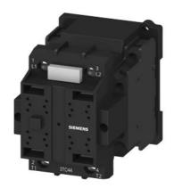
Contactor, Size 2, 2-pole, DC-3 and 5, 32 A Auxiliary contacts 22 (2 NO + 2 NC) 230 V AC 50/60 Hz AC operation
