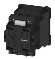
Contactor size 2, 2-pole DC-3 and 5, 32 A Auxiliary switch 22 (2 NO + 2 NC) Alternating current operation 120 V AC 60 Hz/110 V AC 50 Hz
