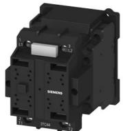
Contactor, Size 2, 2-pole, DC-3 and 5, 32 A Auxiliary contacts 22 (2 NO + 2 NC) 24 V AC 60 Hz/20 V AC 50 Hz AC operation
