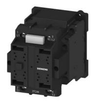
Contactor, Size 2, 2-pole, DC-3 and 5, 32 A Auxiliary contacts 22 (2 NO + 2 NC) 24 V AC 50 Hz/29 V AC 60 Hz AC operation
