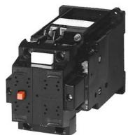
Contactor, Size 2, 2-pole, DC-3 and 5, 32 A Auxiliary contacts 22 (2 NO + 2 NC) 230 V DC DC operation
