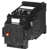
Contactor, Size 2, 2-pole, DC-3 and 5, 32 A, Auxiliary contacts 22 (2NO + 2NC) 250 V DC DC operation
