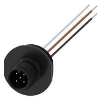
Accessory for position switch Connector plug (5-pole), M12, for M20 x 1.5 for 125 V, 4 A on Pin 5 a yellow/green cable for PE
