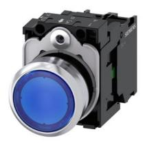
Illuminated pushbutton, 22 mm, round, Metal, shiny, blue, pushbutton, flat, momentary contact type, with holder, 1NO, LED module with integrated LED 230 V AC, screw terminal, with laser labeling, upper case and lower case, always upper case at the beginning of the word
