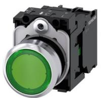
Illuminated pushbutton, 22 mm, round, Metal, shiny, green, pushbutton, flat, momentary contact type, with holder, 1NO, LED module with integrated LED 230 V AC, screw terminal, with laser labeling, symbol number according to, ISO 7000 or IEC 60417
