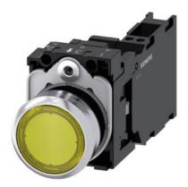
Illuminated pushbutton, 22 mm, round, Metal, shiny, yellow, pushbutton, flat, momentary contact type, with holder, 1 NO+1 NC, LED module with integrated LED 230 V AC, spring-type terminal, with laser labeling, symbol number according to, ISO 7000 or IEC 60417
