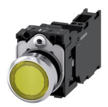
Illuminated pushbutton, 22 mm, round, Metal, shiny, yellow, pushbutton, flat, momentary contact type, with holder, 1 NO+1 NC, LED module with integrated LED 230 V AC, spring-type terminal, with laser labeling, upper case and lower case, always upper case at beginning of line
