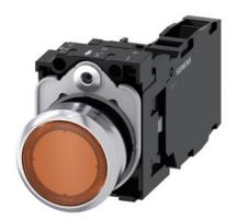
Illuminated pushbutton, 22 mm, round, metal, shiny, amber, pushbutton, flat, momentary contact type, with holder, 1 NO+1 NC, LED module with integrated LED 230 V AC, screw terminal, with laser labeling, upper case
