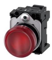
Indicator lights, 22 mm, round, metal, shiny, red, lens, smooth, with holder, LED module with integrated LED 110 V AC, spring-type terminal, with laser labeling, symbol number according to, ISO 7000 or IEC 60417
