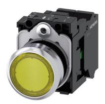
Illuminated pushbutton, 22 mm, round, metal, shiny, yellow, pushbutton, flat, momentary contact type, with holder, 1NO, LED module with integrated LED 110 V AC, spring-type terminal, with laser labeling, upper case
