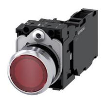
Illuminated pushbutton, 22 mm, round, metal, shiny, red, pushbutton, flat, momentary contact type, with holder, 1 NO+1 NC, LED module with integrated LED 110 V AC, screw terminal, with laser labeling, symbol number according to, ISO 7000 or IEC 60417
