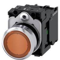
Illuminated pushbutton, 22 mm, round, metal, shiny, amber, pushbutton, flat, momentary contact type, with holder, 1NO, LED module with integrated LED 110 V AC, screw terminal, with laser labeling, upper case
