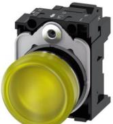
Indicator lights, 22 mm, round, metal, shiny, yellow, lens, smooth, with holder, LED module with integrated LED 24 V AC/DC, spring-type terminal, with laser labeling, inscription or symbol Customer-specific selection with SIRIUS ACT configurator (CIN)
