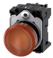
Indicator lights, 22 mm, round, metal, shiny, amber, lens, smooth, with holder, LED module with integrated LED 24 V AC/DC, screw terminal, with laser labeling, lower case
