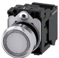
Illuminated pushbutton, 22 mm, round, metal, shiny, clear, pushbutton, flat, momentary contact type, with holder, 1NO, LED module with integrated LED 24 V AC/DC, spring-type terminal, with laser labeling, upper case and lower case, Always upper case at the beginning of the word
