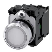
Illuminated pushbutton, 22 mm, round, metal, shiny, white, pushbutton, flat, momentary contact type, with holder, 1NO, LED module with integrated LED 24 V AC/DC, screw terminal, with laser labeling, inscription or symbol Customer-specific selection with SIRIUS ACT configurator (CIN)
