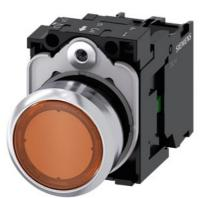
Illuminated pushbutton, 22 mm, round, metal, shiny, amber, pushbutton, flat, momentary contact type, with holder, 1NO, LED module with integrated LED 24 V AC/DC, screw terminal, with laser labeling, upper case
