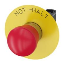
EMERGENCY STOP mushroom-type actuator, 22 mm, round, metal, shiny, red, 40 mm, positive latching, according to EN ISO 13850, pull-to-unlatch mechanism, with yellow backing plate, inscription: NOT-HALT, with holder, 1 NC, 1 NC, spring-type terminal
