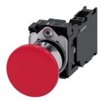
Mushroom pushbutton, 22 mm, round, metal, shiny, red, 40mm, latching, pull-tounlatch mechanism, with holder, 1 NO+1 NC, spring-type terminal, with laser labeling, symbol number according to, ISO 7000 or IEC 60417
