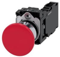
Mushroom pushbutton, 22 mm, round, metal, shiny, red, 40mm, latching, pull-to-unlatch mechanism, with holder, 1 NO+1 NC, screw terminal, with laser labeling, symbol number according to, ISO 7000 or IEC 60417
