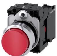
Pushbutton, 22 mm, round, metal, shiny, red, pushbutton, raised, momentary contact type, with holder, 1 NC, screw terminal, with laser labeling, symbol number according to, ISO 7000 or IEC 60417
