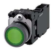
Illuminated pushbutton, 22 mm, round, plastic with metal front ring, green, pushbutton, flat, momentary contact type, with holder, 1 NO+1 NC, LED module with integrated LED 110 V AC, screw terminal, with laser labeling, lower case
