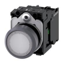
Illuminated pushbutton, 22 mm, round, plastic with metal front ring, white, pushbutton, flat, momentary contact type, with holder, 1NO, LED module with integrated LED 24 V AC/DC, screw terminal, with laser labeling, upper case and lower case, Always upper case at the beginning of the word
