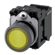
Illuminated pushbutton, 22 mm, round, plastic with metal front ring, yellow, pushbutton, flat, momentary contact type, with holder, 1NO, LED module with integrated LED 24 V AC/DC, spring-type terminal, Z=20-unit packaging
