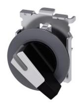
Selector switch, illuminable, 30 mm, round, metal, matte, white, selector switch, long, front ring for flush installation, 2 switch positions O<I, momentary contact type, Actuating angle  $45^\circ$ , 10:30h/12h
