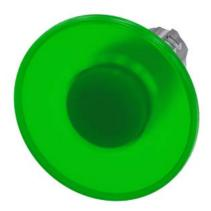
Illuminated mushroom pushbutton, 22 mm, round, metal, shiny, green, 60 mm, latching, pull-to-unlatch mechanism, Z=40-unit packaging
