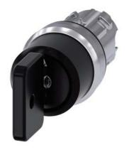
Key-operated switch O.M.R, 22 mm, round, metal, shiny, lock number 73034, black, with 2 keys, 3 switch positions I-O-II, latching, actuating angle 2x45°, 10:30h/12h/13:30h, key removal O, with laser labeling, upper case and lower case, always upper case at beginning of line
